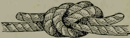
FIG. 19.—Ordinary knot (finished).
